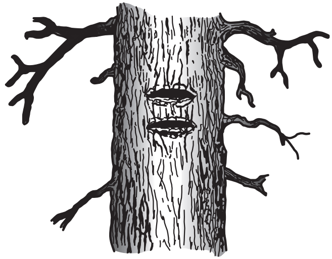
Figure 3-53. Hack marks on a line tree.
